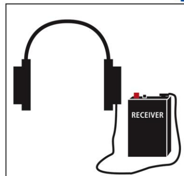
Headset with Receiver Allows wearer to hear clearly within a looped room without the use of a hearing aid.
