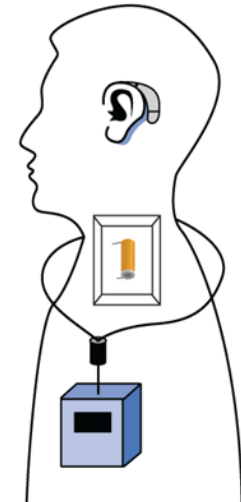
Telecoil inside streamer
