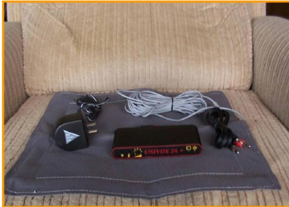
Amplifier plugged into TV just like a room loop with a wire discreetly strung to TV viewing chair and hooked to loop pad that goes under the chair's cushion (can also be used under the mattress in a bed).
