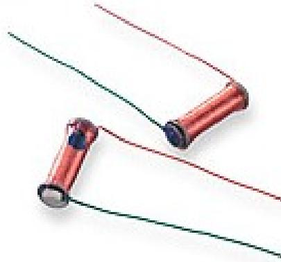
**Telecoils are tiny copper receivers for sound transmitted as an electromagnetic signal.**
